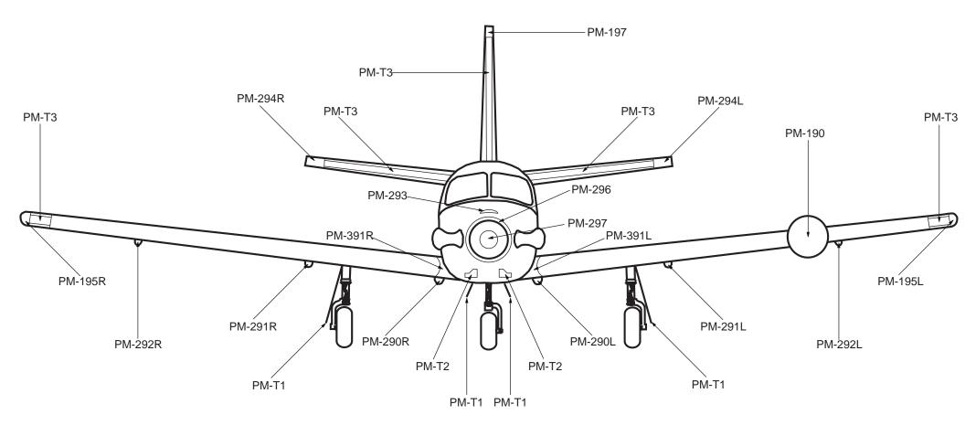
NOTE: All Pre-Formed Protective Masks (Boots) should be installed prior to installing tape.
