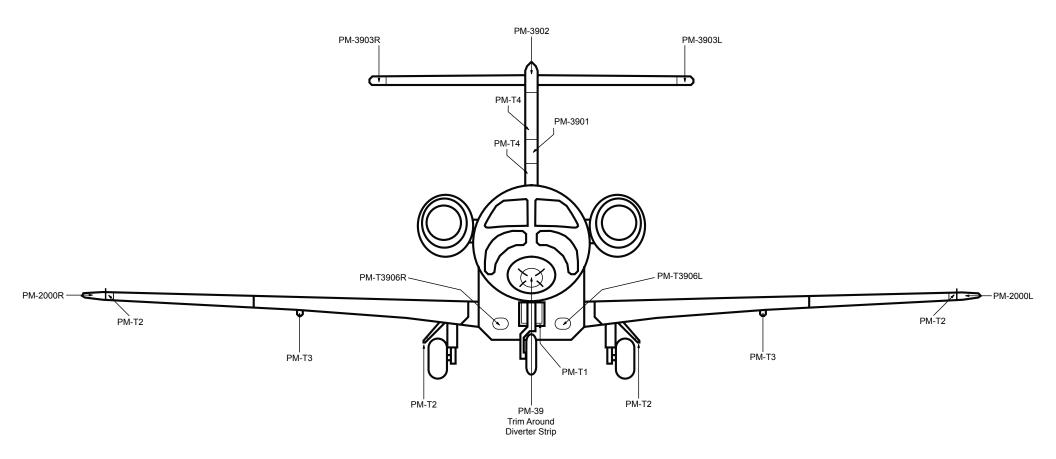
NOTE: All Pre-Formed Protective Masks (Boots) should be installed prior to installing tape.
